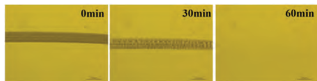
Figure 10. Optical microscope images of self-healing behavior of scratched cross-linked hybrid film PI@POSS-AN/1-1 at 150 °C. Scale bar is 100 \mu\text{m} .
