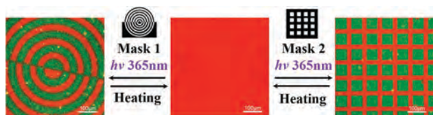
Figure 9. CLSM images of photo-rewritable fluorescence micro-pattern which were prepared on sample PI@POSS-AN/1-1, alternately overlay/removing masks (“grid” and “annulus”) under 365 nm UV illumination. Erasure procedure was achieved by heating the patterned film at 150 °C for 1 h. The excitation wavelength of blue light for CLSM is fixed at 404 nm.
